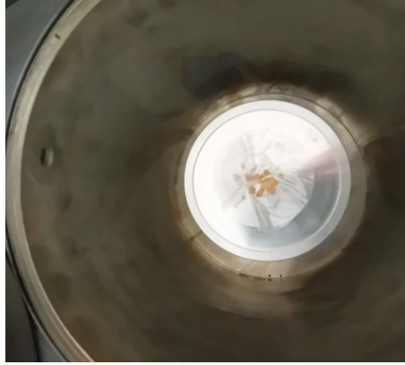
FIGURE 9.5.1. The placement of our thorium-containing sample material in the lead shielded HPGe detector.
