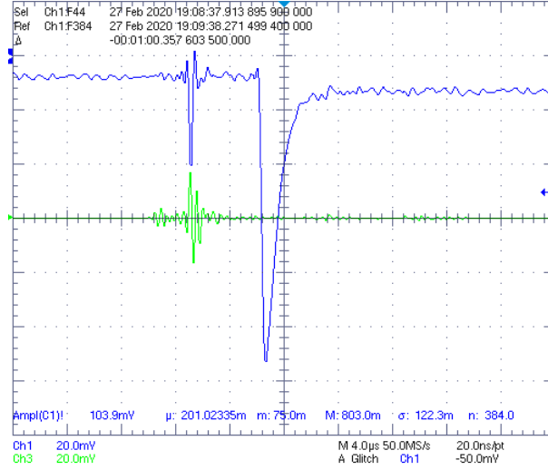
FIGURE 6.8.4. An exemplary oscillogram. The blue curve is the PhEM signal, and the green curve is the radio antenna signal. The large negative dip is the signature of a gamma ray quantum.
