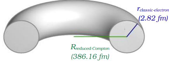
FIGURE 3.3.1. An illustration of the electron's particle aspect. The electric current circulates at the speed of light within a torus whose major radius is the reduced Compton radius, and whose minor radius is classical electron radius. This circular Zitterbewegung motion generates the electron's spin.
